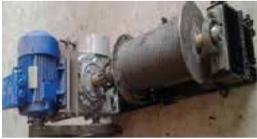
WIRE PULLING MACHINE (BIG HOIST)
