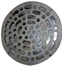
MS SCREEN INSIDE REACTOR
