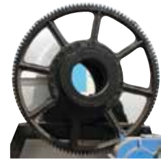
118 TEETH MAIN REACTOR BIG GEAR (CHAKKAR)
