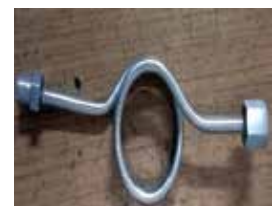
SIFON PIPE FOR PRESSURE SENSOR
